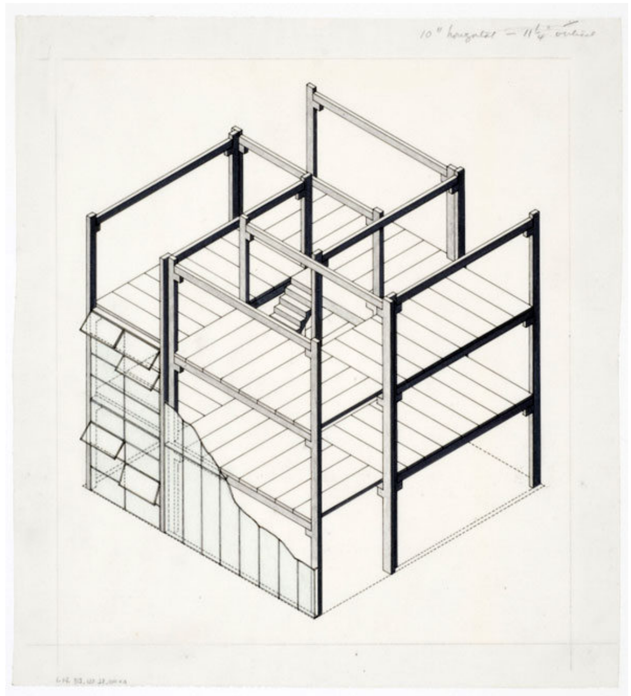
James Frazer Stirling. Stiff Dom-ino Housing, theoretical project (1951) cut-away axonometric view with hinged windows
